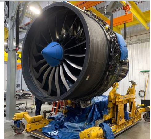
Westmont's Gantry System removing an engine from a shipping stand.
